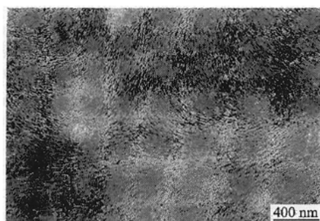
Fig. 5 TEM microphotographs of lamellar structure crystallized from the nematic glassy state of Pd-10 polymer after annealing at 90°C for 2 h, stained by RuO 4
